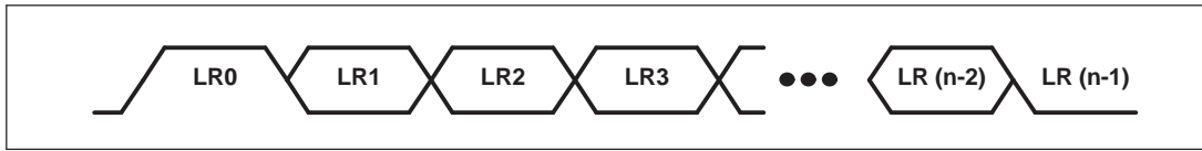
Each cell represents one clock sample period, and n is the number of bits in the request stream.
