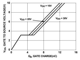
Figure 7. Gate Charge Characteristics
