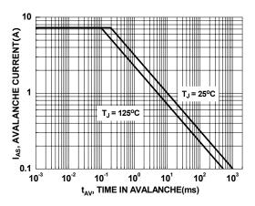
Figure 9. Unclamped Inductive Switching Capability
