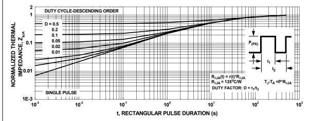
Figure 13. Transient Thermal Response Curve
