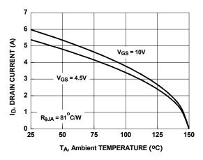
Figure 10. Maximum Continuous Drain Current vs
