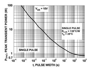
Figure 12. Single Pulse Maximum Power Dissipation
