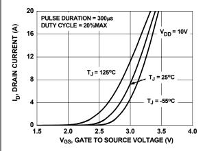
Figure 5. Transfer Characteristics
