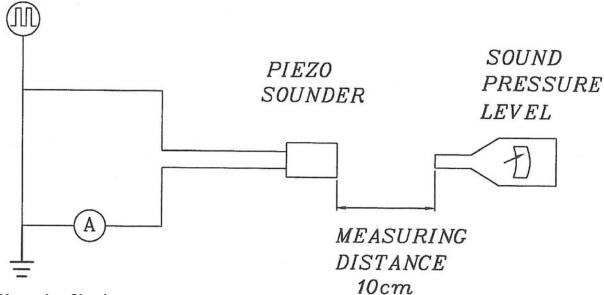
S.P.L. Measuring Circuit Input Signal: 10 Vp-p, 4.0 KHz, Square Wave
