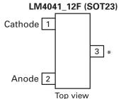
\* Pin 3 must be left floating or connected to pin 2
