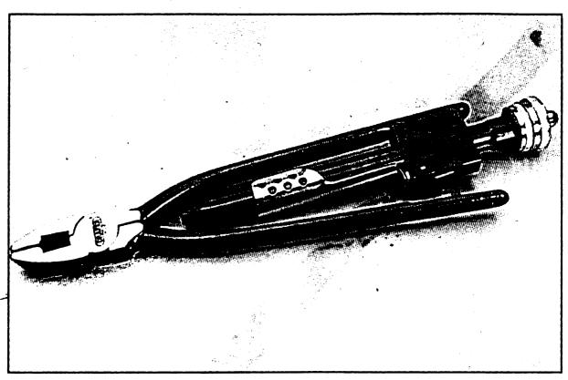
Mainly used in the aero and defence industries for wire tying knots. Manufactured from chrome vanadium steel hardened, tempered with painted handles and chrome plated spiral screw assembly. Plier faces polished. Overall length 250mm. Display packed.
