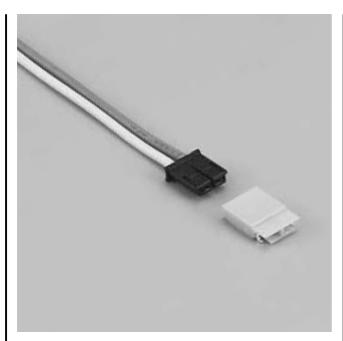
Low profile connector with high withstanding voltage, designed for connecting liquid crystal display backlight lamps to their starters. The BHL connector is 2.8mm (.110") thick, so the mounting height is only 3mm (.118").
