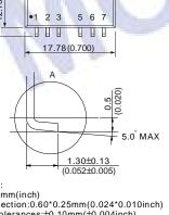
Pin tolerances:±0.10mm(±0.004inch) General tolerances: ±0.25mm(±0.010inch)
