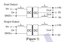
It should also be noted that the inductance and the frequency of the "LC" filtering network should be staggered with the DC/DC frequency to avoid mutual interference. However, the capacitance of the output filter capacitor must be proper. If the capacitance is too big, a startup problem might arise. For every channel of output, provided the safe and reliable operation is ensured, the recommended capacitance of its filter capacitor sees (Table 1).
