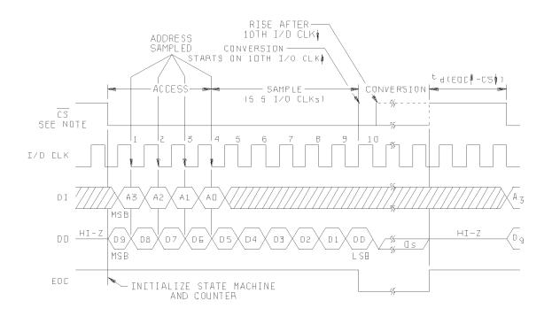
NOTE: To minimize errors caused by noise at  $\overline{\text{CS}}$ , the internal circuitry waits for a setup time after  $\overline{\text{CS}} \downarrow$  before responding to control input signals. No attempt should be made to clock in input data until the minimum  $\overline{\text{CS}}$  setup time elapses.
