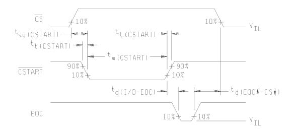
FIGURE 4. Switching waveforms and test circuit - Continued.
