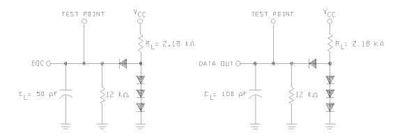
NOTE:  $C_L$  includes probe and jig capacitance.
