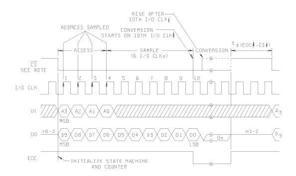
NOTE: To minimize errors caused by noise at  $\overline{\text{CS}}$ , the internal circuitry waits for a setup time after  $\overline{\text{CS}}$  ↓ before responding to control input signals. No attempt should be made to clock in input data until the minimum  $\overline{\text{CS}}$  setup time elapses.
