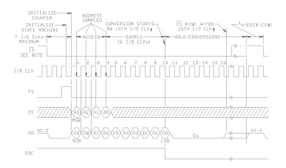
NOTE: To minimize errors caused by noise at  $\overline{\text{CS}}$ , the internal circuitry waits for a setup time after  $\overline{\text{CS}}$  ↓ before responding to control input signals. No attempt should be made to clock in input data until the minimum  $\overline{\text{CS}}$  setup time elapses.
