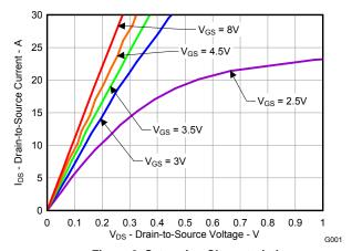
Figure 2. Saturation Characteristics
