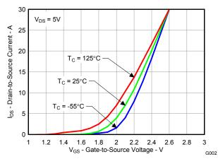
Figure 3. Transfer Characteristics
