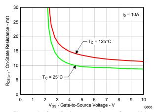
Figure 7. On-State Resistance vs. Gate-to-Source Voltage
