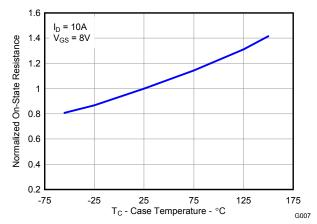
Figure 8. Normalized On-State Resistance vs. Temperature
