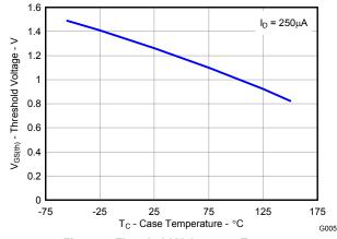
Figure 6. Threshold Voltage vs. Temperature
