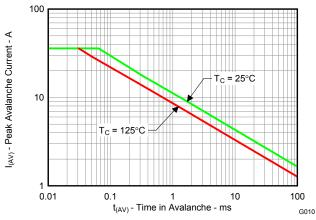
Figure 11. Single Pulse Unclamped Inductive Switching
