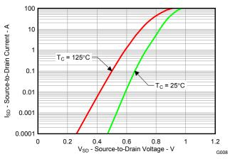
Figure 9. Typical Diode Forward Voltage
