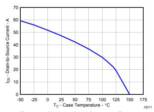
Figure 12. Maximum Drain Current vs. Temperature
