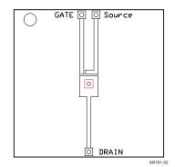
Max  $R_{\theta JA} = 165^{\circ} C/W$  when mounted on a minimum pad area of 2-oz. (0.071-mm thick) Cu.
