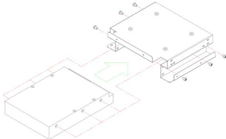
4. Secure the CD-ROM on the 3-in-1 drive bay after fastening it onto a transfer card.
