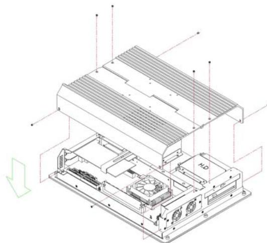
2. Remove the 3-in-1 drive bay in accordance with the picture.
