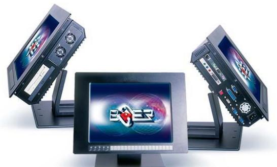
The BPC-6670 is a 15" industrial Panel PC built around the Intel® Pentium® 4 CPU with clock rate 2.4GHz/2.8GHz and 400MHz FSB/533MHz FSB. The rear design of BPC-6670 enhances the disassembly process when required. It also supports various mounting solutions like wallmount, or desktop for different applications.
