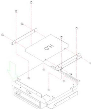
6. The fully-equipped, 3-in-1 drive bay is placed on the BPC-6670 by means of screw.
