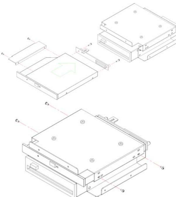
5. Fasten the 2.5-inch HDD onto the 3-in-1 drive bay.
