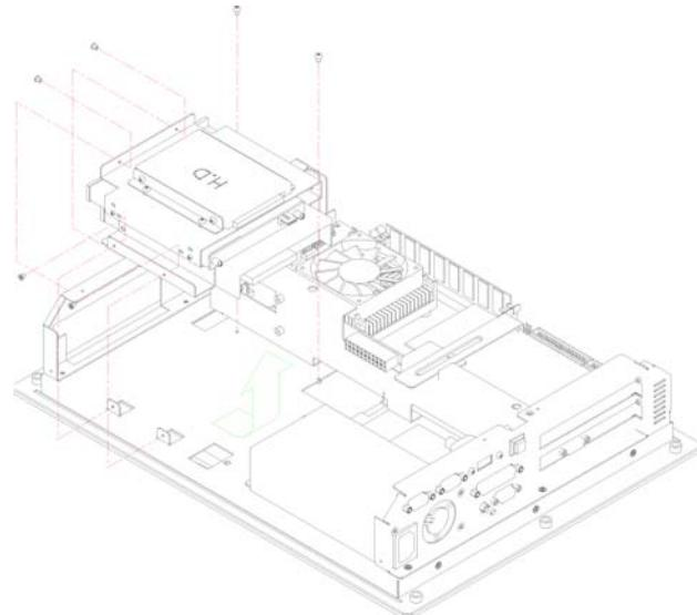
3. The 3.5-inch FDD (or the 3.5-inch HDD) is installed on top of the 3-in-1 drive bay.
