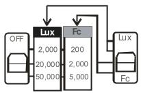
Example: If a measurement on the 5000 Fc range displays 350, then the actual measured value is;  $350 \times 10 = 3500$  Fc.
