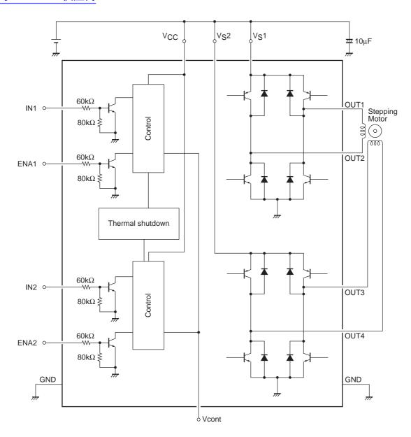
\*: As long as the voltages applied to  $V_{CC}$ ,  $V_{S1}$ ,  $V_{S2}$ , ENA1, ENA2, IN1 and IN2 are within the limits set by the absolute maximum ratings, there are no restrictions on the relationship of each voltage level in comparison with the others (regarding which is higher or lower). (ex.  $V_{CC} = 3V$ ,  $V_{S1}$
