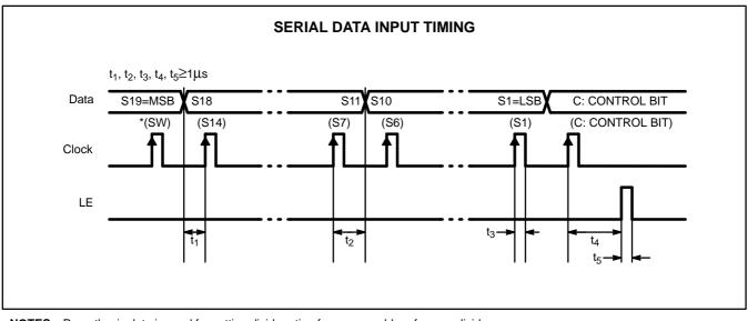
**NOTES:** Parenthesis data is used for setting divide ratio of programmable reference divider. On rising edge of clock shifts one bit of data into the shift register.
