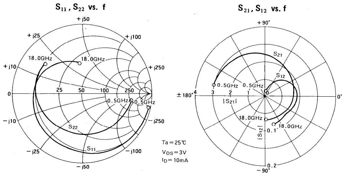
S PARAMETERS (Ta = 25°C, V<sub>DS</sub> = 3V, I<sub>D</sub> = 10mA)
