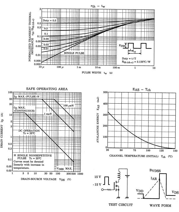
$R_{G} = 25 \Omega$  $EAS = \frac{1}{2} \cdot L \cdot I^2 \cdot \left(\frac{B_{VDSS}}{B_{VDSS} - V_{DD}}\right)$ V<sub>DD</sub> = 90 V, L = 3.83 mH
