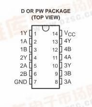
The SN74HC02 contains four independent 2-input NOR gates. It performs the Boolean function  $Y = \overline{A} + \overline{B}$  or  $Y = \overline{A} \cdot \overline{B}$  in positive logic.
