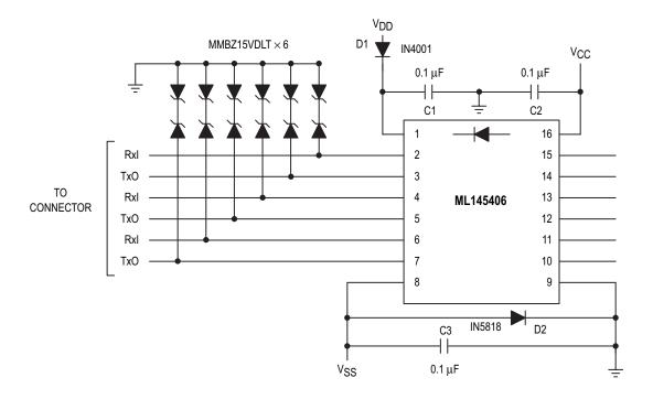
Figure 4. ESD and Power Supply Networks
