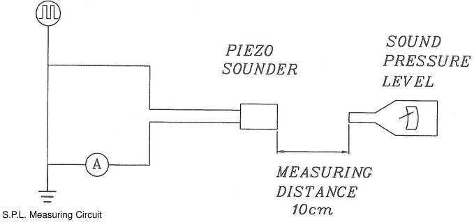
Input Signal: 10 V p-p, 2.5 KHz, Square Wave
