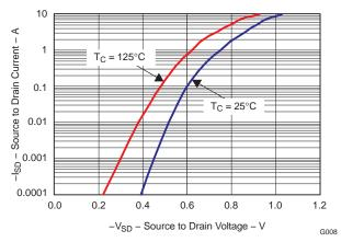
Figure 9. Typical Diode Forward Voltage
