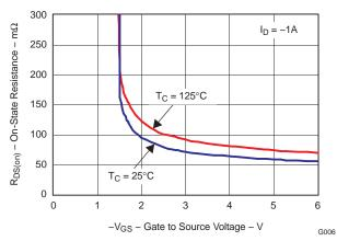
Figure 7. On Resistance vs. Gate Voltage
