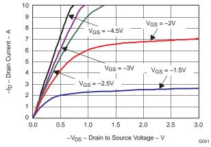
Figure 2. Saturation Characteristics
