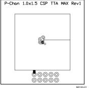
Max  $R_{\theta JA} = 105^{\circ}\text{C/W}$  when mounted on 1 inch<sup>2</sup> of 2 oz. Cu.
