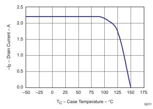
Figure 11. Maximum Drain Current vs. Temperature
