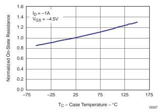
Figure 8. On Resistance vs. Temperature
