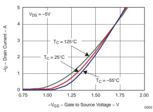
Figure 3. Transfer Characteristics
