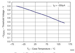
Figure 6. Threshold Voltage vs. Temperature
