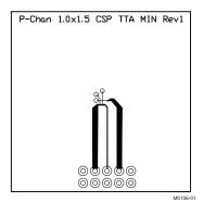
Max  $R_{\theta JA} = 270^{\circ} C/W$  when mounted on minimum pad area of 2 oz. Cu.
