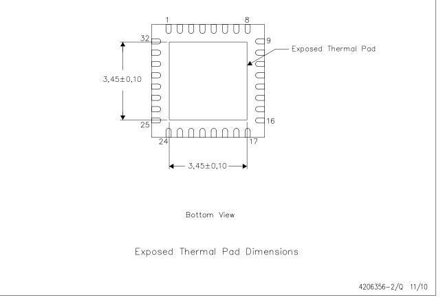
NOTE: A. All linear dimensions are in millimeters
