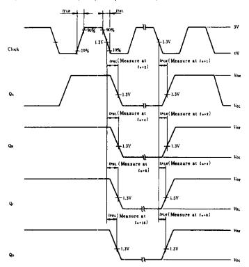
Notes) 1. Input pulse:  $t_{TLH} \le 15$ ns,  $t_{THL} \le 5$ ns, PRR=1MHz, duty cycle=50% and: for  $f_{max}$ ,  $t_{TLH} = t_{THL} \le 2.5$ ns.
