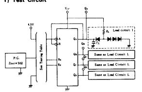
Notes) 1.  $C_L$  includes probe and jig capacitance.
