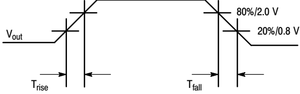
Figure 14. Waveforms: Rise and Fall Times
