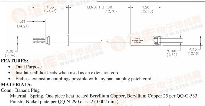
Insulation: Polypropylene, molded to plug body and wire. Color matches color of wire.
