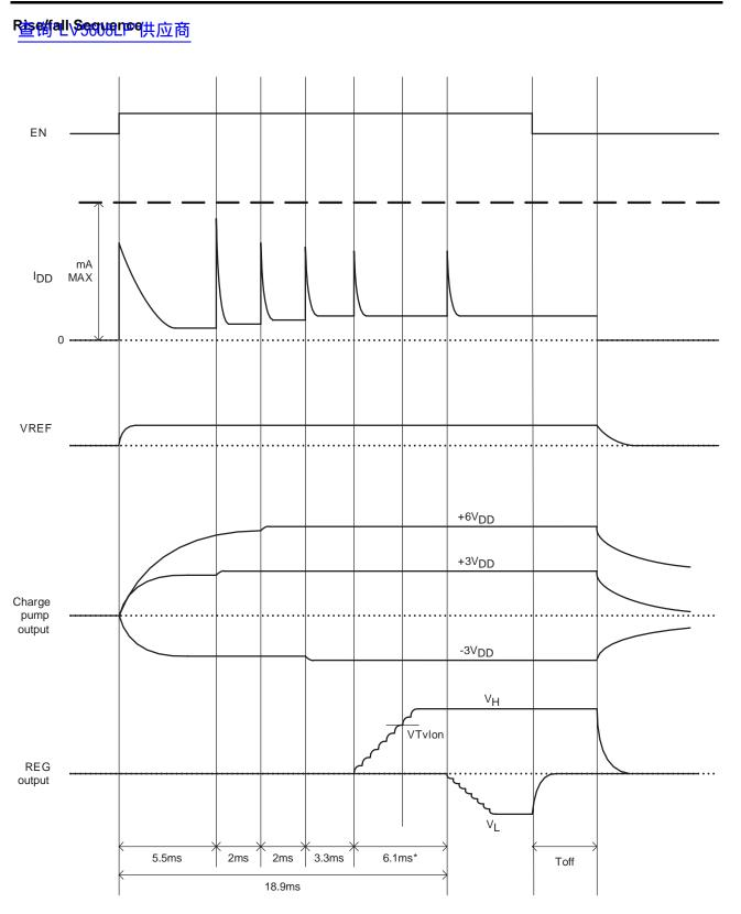
\*The VL startup time at VH  $\ge$  10V and after elapse of 6.1ms is the reference time for CLK = 2MHz.
