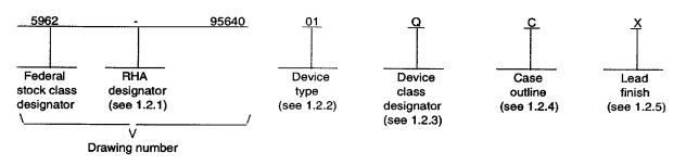
1.2.1 <u>RHA designator</u>. Device classes N, Q, and V RHA marked devices meet the MIL-PRF-38535 specified RHA levels and are marked with the appropriate RHA designator. Device class M RHA marked devices meet the MIL-PRF-38535, appendix A specified RHA levels and are marked with the appropriate RHA designator. A dash (-) indicates a non-RHA device.
