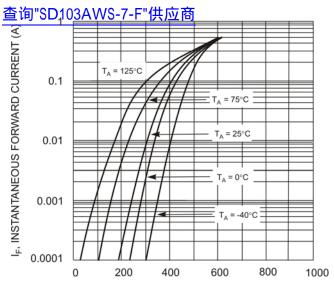
V<sub>F</sub>, INSTANTANEOUS FORWARD VOLTAGE (mV) Fig. 1 Typical Forward Characteristics
