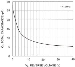
Fig. 3 Typ. Total Capacitance vs. Reverse Voltage
