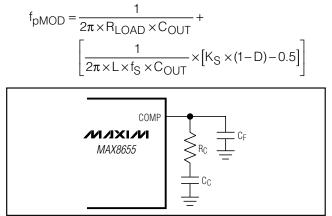
Figure 9. Compensation Components
