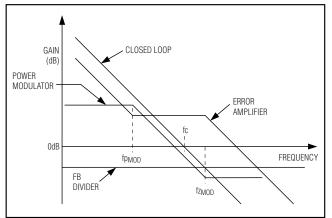
Figure 10. Simplified Gain Plot for the f<sub>ZMOD</sub> > f<sub>C</sub> Case
