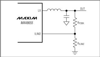
Figure 7. ILIM2 Resistor Connections
