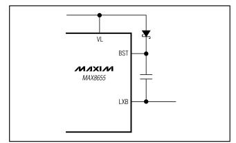
Figure 2. High-Side Gate Boost Circuit
