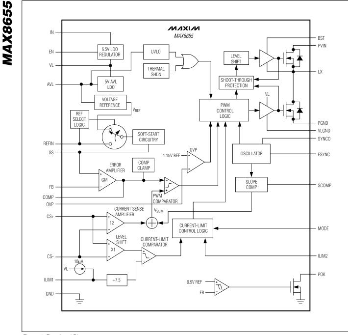
Figure 1. Functional Diagram
