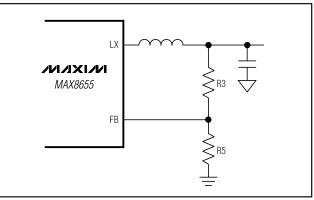
Figure 5. Setting the Output Voltage with a Resistor Voltage-Divider
