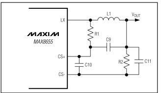
Figure 8. Current Sense Using the Inductor's DC Resistance
