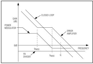
Figure 11. Simplified Gain Plot for the f<sub>ZMOD</sub> < f<sub>C</sub> Case
