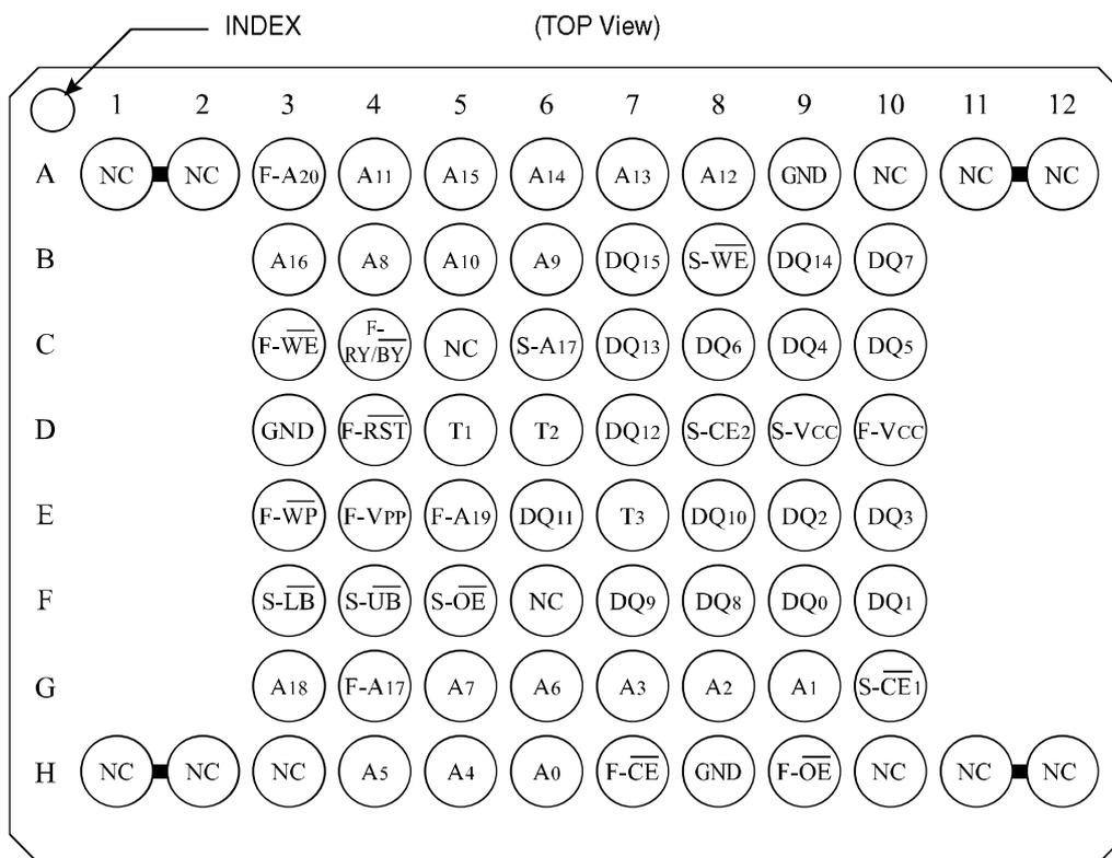
Note) From T1 to T3 pins are needed to be open.
