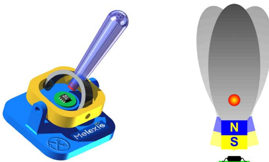
Figure 3 - Typical application of MLX90333
