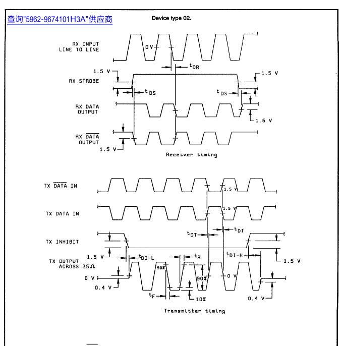
NOTE: Both inputs "TX DATA IN" and "TX DATA IN" must be in the same logic states during off times.
