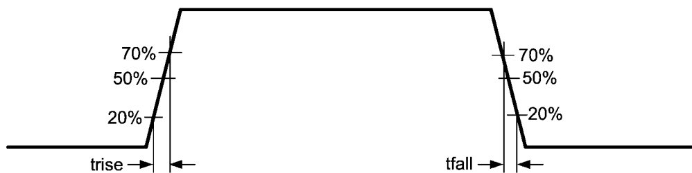
FIGURE 2. Output Transition Time (A and B Side)
