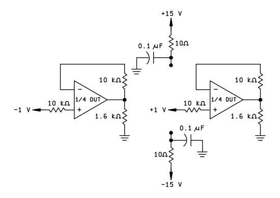
FIGURE 2. Radiation exposure circuit.
