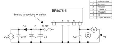
For actual usage, Please kindly evaluate and confirm our part mounted in your product, Especially, Please make sure to confirm whether the load current exceed Max. rated current by using the current probe.
