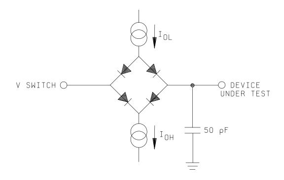
FIGURE 3. Switching test circuit and waveforms.
