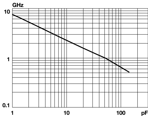
Typical Self Resonant Frequency vs. Capacitance Accu-F®/Accu-P® 0805
