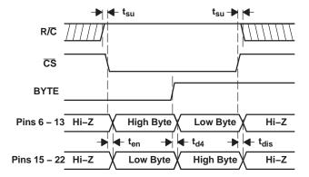
Figure 25. Using CS and BYTE to Control Data Bus
