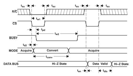
Figure 24. Using CS to Control Conversion and Read Timing
