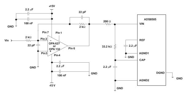
Figure 27. Typical Driving Circuit (±10 V, No Trim)
