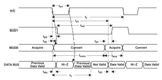
Figure 23. Conversion Timing with Outputs Enabled after Conversion (CS Tied Low)
