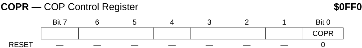
Figure 5-1. COP Control Register
