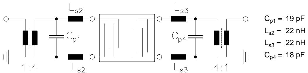
Transformers are only required for measurement in a 50  $\Omega$  environment.
