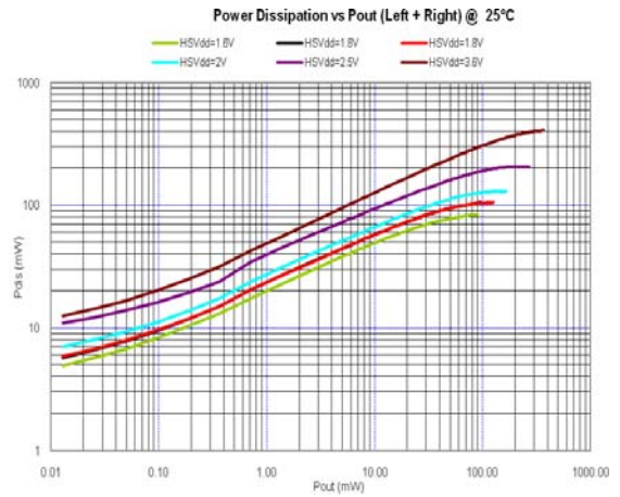
Figure 16. Power Dissipation vs P_{out} with 16\ \Omega Load
