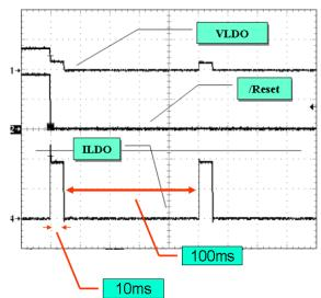
Figure 15. LDO Converter Overcurrent Protection
