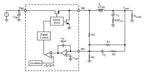
Figure 29. Buck Regulator Control Circuit
