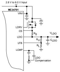
Figure 31. 34702 Linear Regulator Circuit
