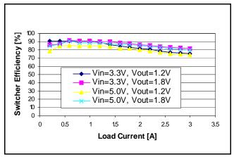
Figure 7. Switcher Efficiency vs. Load Current
