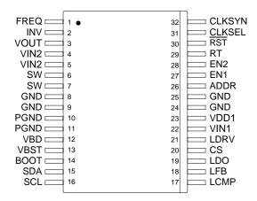
Figure 3. Pin Connections
