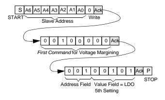
Figure 27. Data Transfer Example - LDO Voltage Margining
