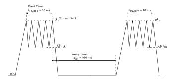
Figure 13. Switching Regulator Current Limit (Not To Scale)
