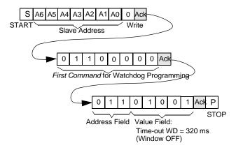
Figure 26. Data Transfer Example - Watch Dog Timer Setting.
