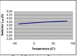
Figure 8. Switcher I<sub>LIM</sub> vs. Temperature
