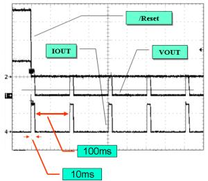
**Figure 14. Switching Converter Overcurrent Protection**
