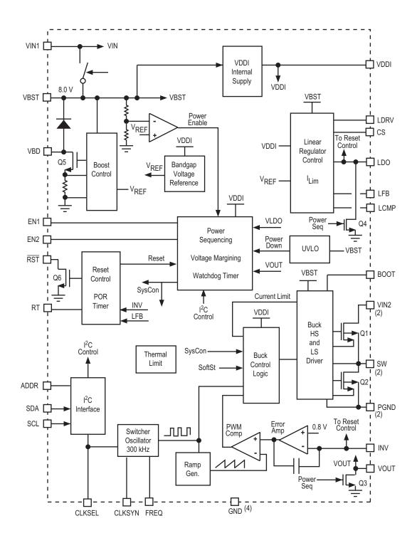
Figure 2. 34702 Simplified Internal Block Diagram
