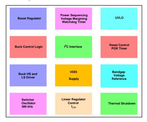
Figure 11. 34702 Functional Internal Block Diagram
