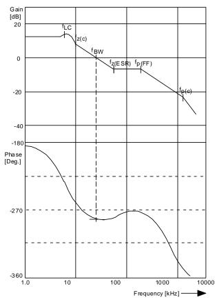
Figure 30. Buck Control Loop Bode Plot
