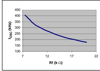
Figure 6. f<sub>OSC</sub> vs. Rf
