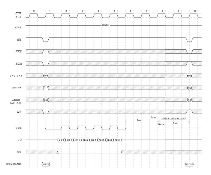
Note 1. The row active command of the precharge bank can be issued after t<sub>RP</sub> from this point. The new read/write command of another activated bank can be issued from this point.
