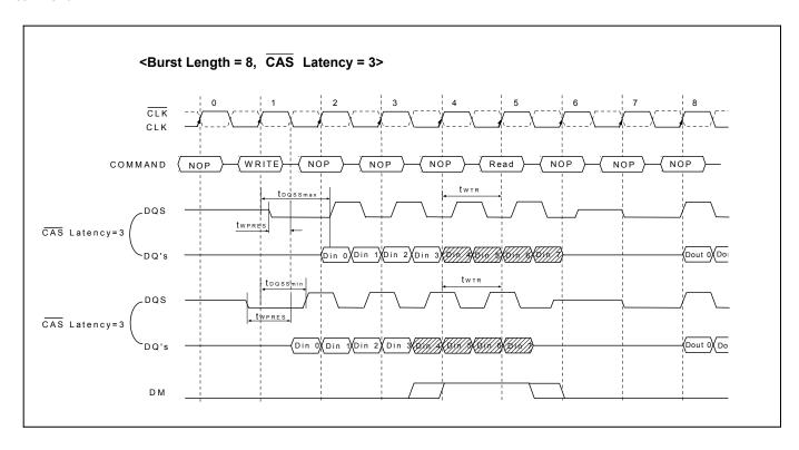
The following functionality established how a Read command may interrupt a Write burst and which input data is not written into the memory.
