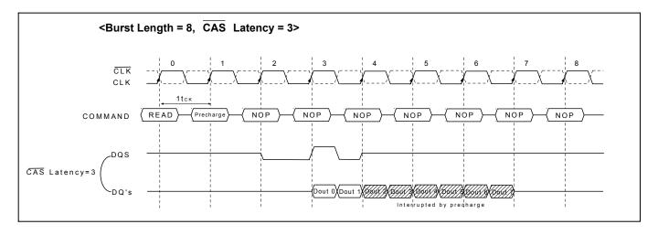
When a burst Read command is issued to a DDR SDRAM, a Precharge command may be issued to the same bank before the Read burst is complete. The following functionality determines when a Precharge command may be given during a Read burst and when a new Bank Activate command may be issued to the same bank.
