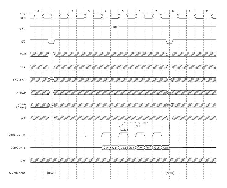
Note 1. The row active command of the precharge bank can be issued after t<sub>RP</sub> from this point. The new read/write command of another activated bank can be issued from this point. At burst read/write with auto precharge, CAS interrupt of the same bank is illegal.
