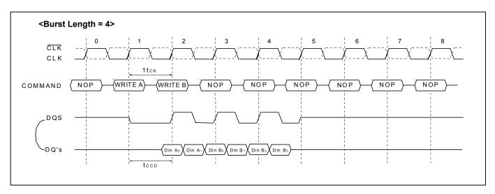
The following functionality establishes how a Write command may interrupt a Read burst.
