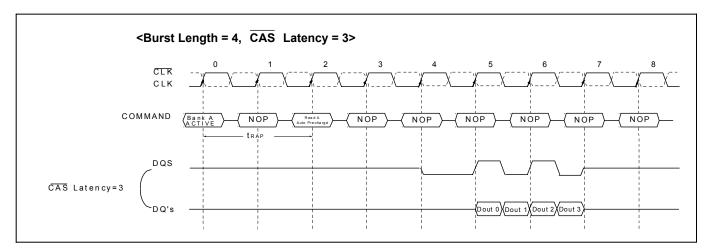
At burst read / write with auto precharge,  $\overline{\text{CAS}}$  interrupt of the same bank is illegal.
