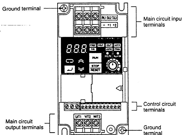
Arrangement of Control Circuit Terminals
