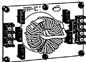
The Simple Input Noise Filter is connected to the power input side to eliminate the noise in the power line connected to the Inverter and suppress noise leaking from the Inverter to the power line.
