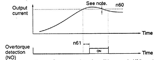
Note: Overtorque detection will be canceled if the output current decreases from the detection level by approximately 5% of the Inverter rated current.
