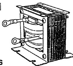
The DC Reactor suppresses harmonic current generated from the Inverter and improves the power factor of the Inverter. The DC Reactor suppresses harmonic current more effectively than the AC Reactor. Furthermore, the DC Reactor can be used in combination with the AC Reactor. Used with either 3-phase or single-phase 200-V AC Inverters.
