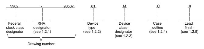
1.2.1 RHA designator. Device classes Q and V RHA marked devices meet the MIL-PRF-38535 specified RHA levels and are marked with the appropriate RHA designator. Device class M RHA marked devices meet the MIL-PRF-38535, appendix A specified RHA levels and are marked with the appropriate RHA designator. A dash (-) indicates a non-RHA device.
