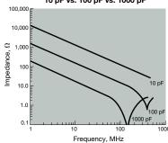
Variation of Impedance with Chip Size Impedance vs. Frequency 1000 pF - C0G (NP0)
