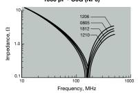
Variation of Impedance with Ceramic Formulation Impedance vs. Frequency 1000 pF - C0G (NP0) vs X7R
