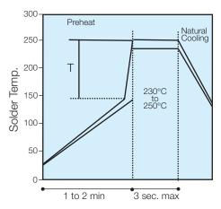
(Preheat chips before soldering) T/maximum 150°C
