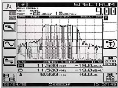
Reverse digital modem signal
