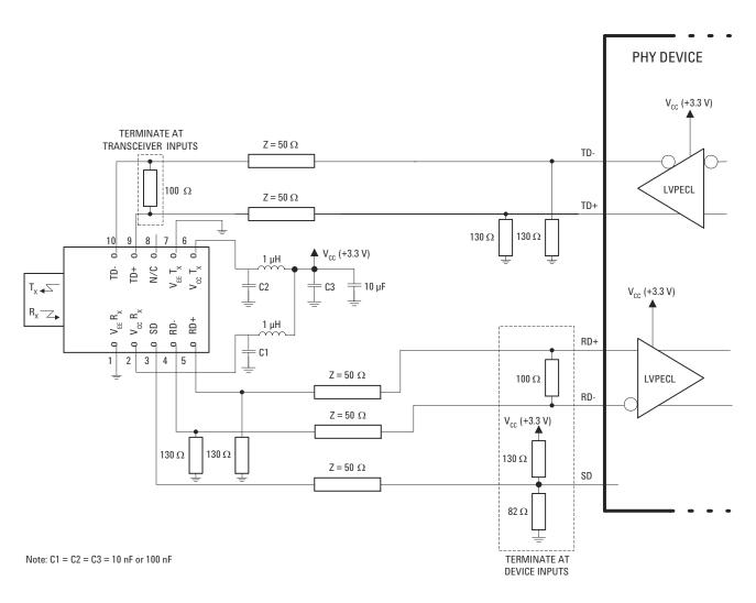
Figure 7. Recommended Decoupling and Termination Circuits
