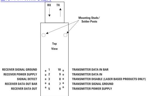
Figure 3. Pin Out Diagram.
