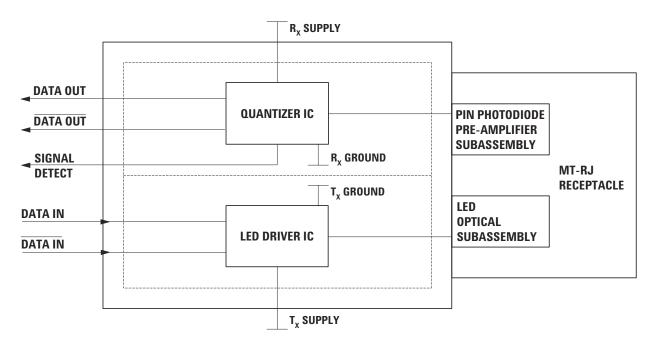
Figure 1. Block Diagram.
