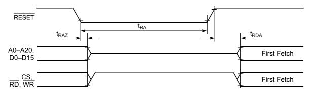
Figure 4-12 Asynchronous Reset Timing
