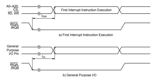
Figure 4-14 External Level-Sensitive Interrupt Timing
