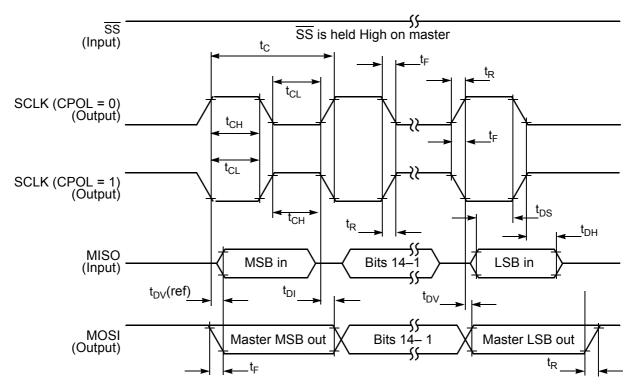
Figure 4-25 SPI Master Timing (CPHA = 1)
