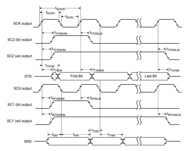
**Figure 4-29 Master Mode Timing Diagram**
