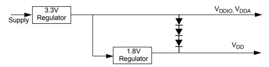
Figure 4-3 Example Circuit to Control Supply Sequencing
