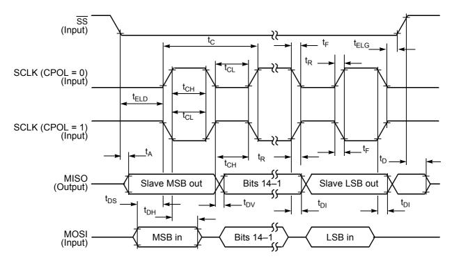
Figure 4-26 SPI Slave Timing (CPHA = 0)
