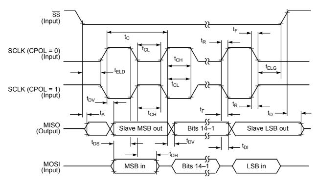
Figure 4-27 SPI Slave Timing (CPHA = 1)
