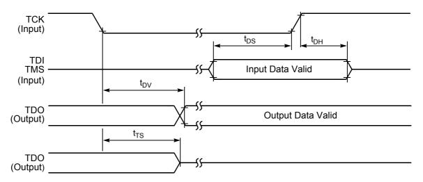
Figure 4-34 Test Access Port Timing Diagram
