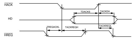
Figure 4-21 Host-to-Controller DMA Write Mode
