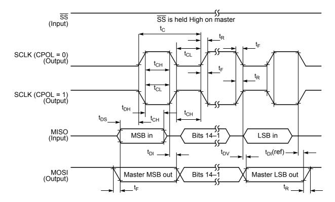
Figure 4-24 SPI Master Timing (CPHA = 0)
