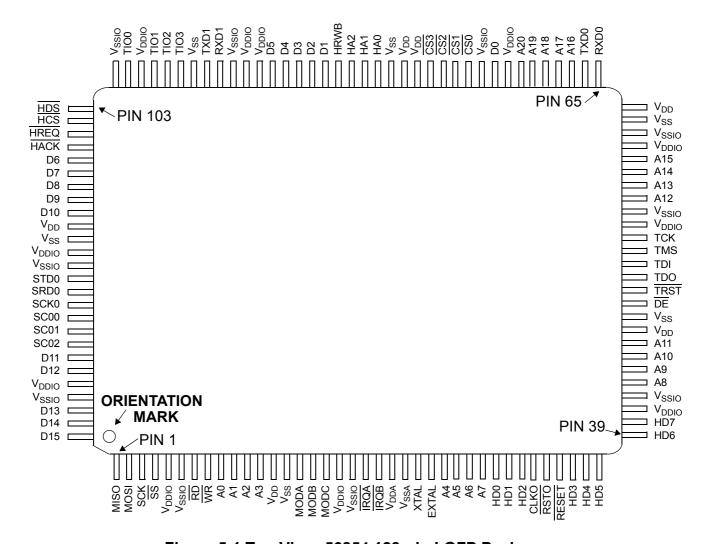
Figure 5-1 Top View, 56854 128-pin LQFP Package
