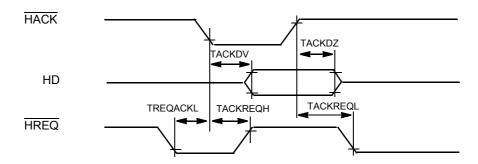
Figure 4-18 Controller-to-Host DMA Read Mode
