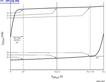
I1 = Charge Pump Sink Current at  $V_{CPout} = Vcc - \Delta V$
