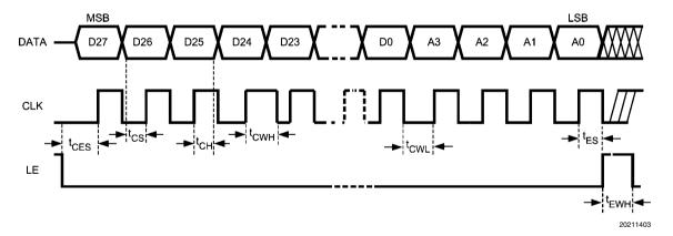
Data bits set on the DATA signal are clocked into a shift register, MSB first, on each rising edge of the CLK signal. On the rising edge of the LE signal, the data is sent from the shift register to the addressed register determined by the LSB bits. After the programming is complete the CLK, DATA, and LE signals should be returned to a low state.
