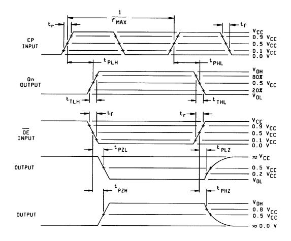
FIGURE 4. Switching waveforms and test circuit.
