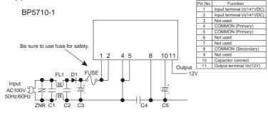
For acutual usage, Please kindly evaluate and confirm our part mounted in your product, Especially, Please make sure to confirm whether the load current exceed Max. rated current by using the current probe.
